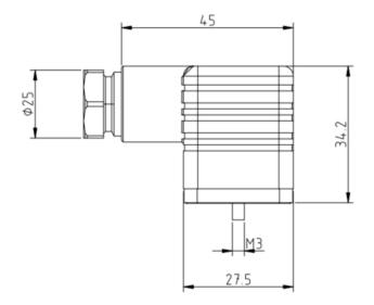
Central Screw Torque value: [50-60] Ncm Hex Nut Torque value: [250-375] Ncm
